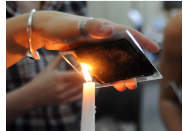
cathode: carbon coating with candle fumes
