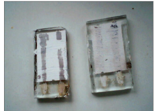
TiO 2 coating after baking with a heat gun
