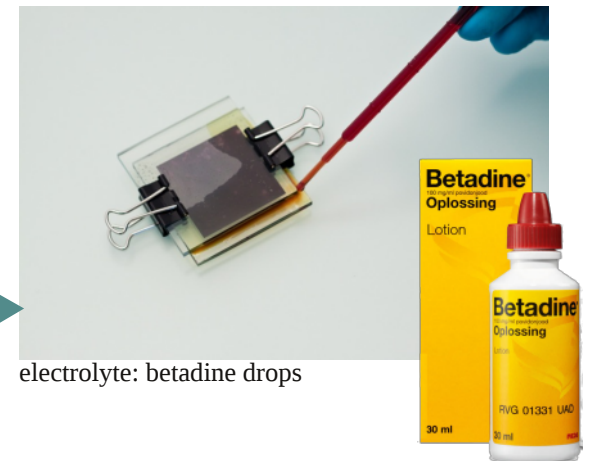
cathode: carbon coating with candle fumes
