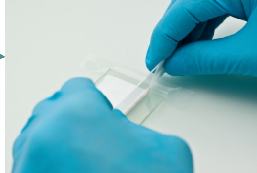
coating with TiO 2 paste
