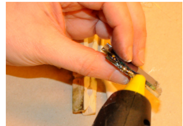
sealing the cells with glue gun (not a permanent solution)
