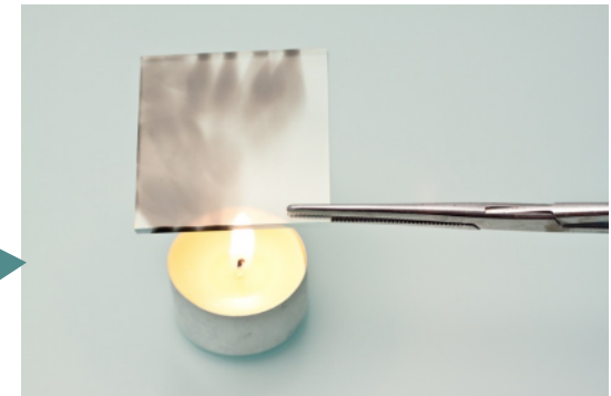
cathode: carbon coating with candle fumes
